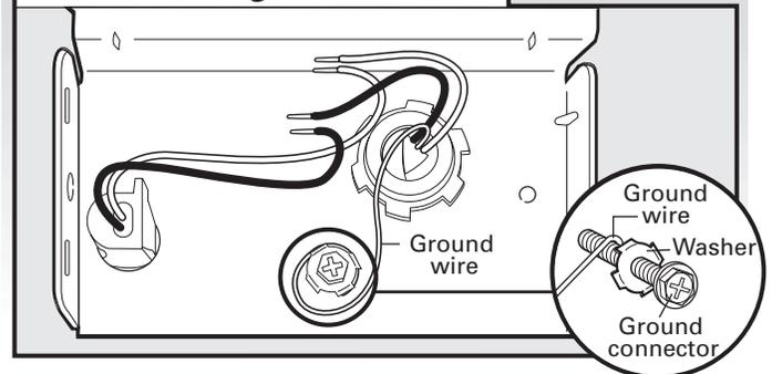
Remove the green grounding screw and place through the ring terminal of the green ground wire. Reattach and tighten the green screw.
